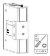
7. Grounding the Device. Grounding will help to prevent the noise effect due to electromagnetic interference (EMI). Connect the device to the site ground wire by the grounding screw before powering on.
