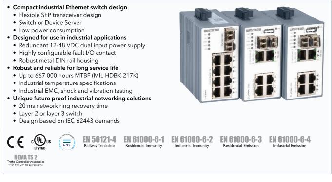
The Lynx 100 and 200 series consists of layer 2 or layer 3 industrial Ethernet switches, powered by WeOS, the Westermo network operating system. The Lynx switches are the most compact switches or device servers on the market, available with up to 10 Ethernet ports whereof two are 100 Mbit or Gbit SFP transceivers.
