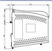
Dimension W x H x D  $34 \times 123 \times 121 \text{ mm} (1.33 \times 4.84 \times 4.76)$
