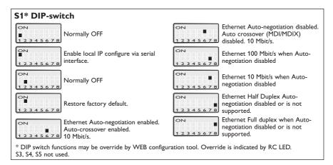
**Note!** DIP-switch alterations are only effective after a power on.
