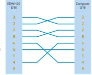
2. Setting DIP S1:1 to 'On' and power-up the EDW-120 this will enable the local IP address to be configured via serial interface.
