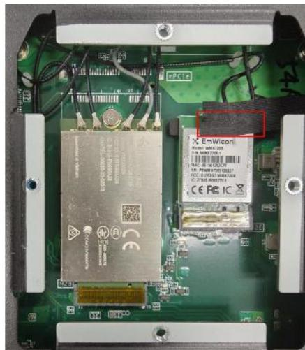
9. Take out the other aluminum block, peel off the blue protective film to expose the adhesive side of the aluminum block, align it with the marked area (red box) on the back of the wireless module door, and firmly press it into place. The adhesive side should face downward to attach the block securely to the module door.
