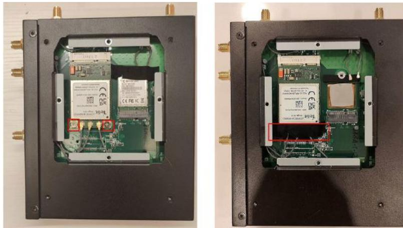
8. Take out the thicker alumin block, peel off the blue protective film to expose the adhesive side of the aluminum block, align it with the marked area (red box) on back of the wireless module door and firmly press it into place. The adhesive side should face downward to attach the block securely to the module door.
