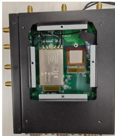
7. Insert the Wi-Fi modem into the M.2 slot. Then, connect the antenna cables to the corresponding modem connectors as shown in the diagram:
