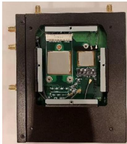
6. Insert the cellular modem into the mPCIe slot. Then, connect the antenna cables to the corresponding modem connectors as shown in the diagram:
