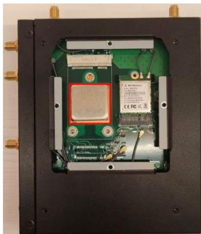
4. Take out the one of the thermal pad. It has two protective films: one blue and one clear. The clear film covers the adhesive side, which should be attached to the aluminum block.
