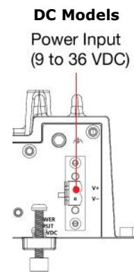
When using AC power, first ensure that you connect the AC power cord to a socket-outlet with earthing connection and use the standard C16 AC inlet along with a C15 plug (refer to the figure in the "Powering On/Off the EXPC-F2000W" section) or standard C15 plug with AC adapter cable. When using DC power, use at least a 100 W power adapter connected through the 2-pin terminal block in the accessories package. The pin assignments for the DC models are shown in the following diagram:
