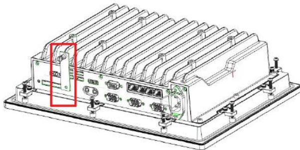
2. Slide the cover to access the slot and insert the CFexpress card into the slot and push it all the way into the slot.
