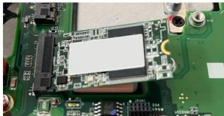
6. Fasten the SSD card in place and secure it by fastening the screw on the socket.
