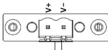
A terminal block is available in the accessories package. The required wire size is 12-14 AWG (Wire Type: Cu, Field Wiring: 2) and a torque value 0.5 N·m (4.5 lb-in) should be applied. The input terminal block should be wired and installed by a skilled person.
