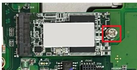
5. Insert an SSD card into the socket or replace the existing one.
