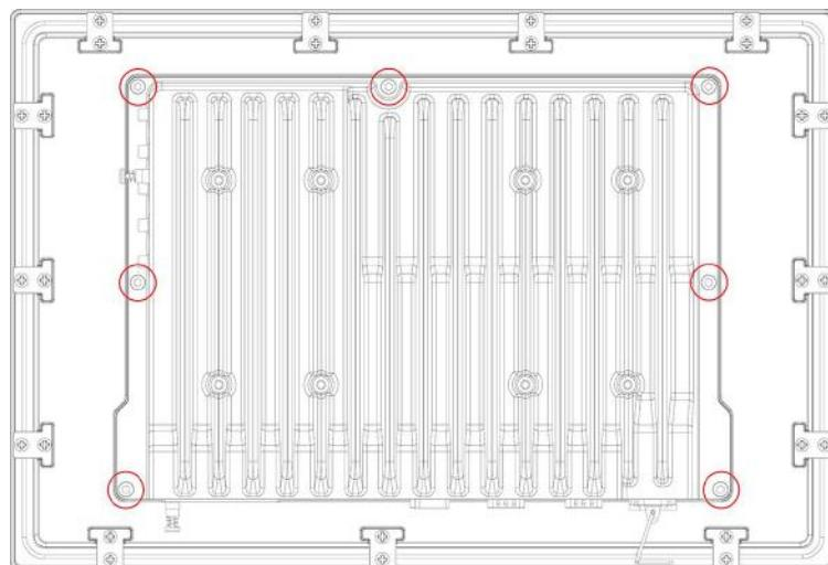
2. Take off the back component of the computer from the panel and remove these ten screws.
