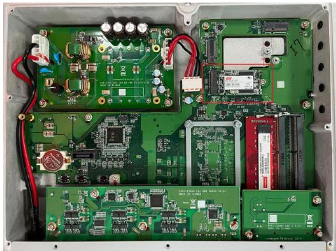
4. If the SSD has already been installed, remove the screw on the end, and remove the SSD.
