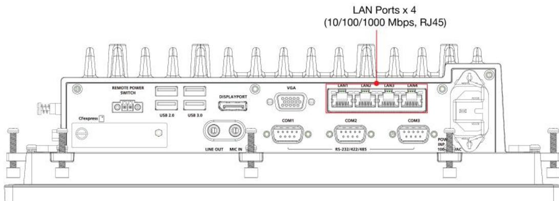
The 10/100/1000 Mbps Ethernet LAN port uses 8-pin RJ45 connectors. The following diagram shows the pinouts and the descriptions for these ports.
