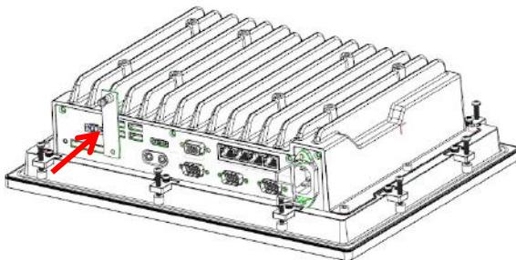
To remove the card, you need to push the card in to release the card.
