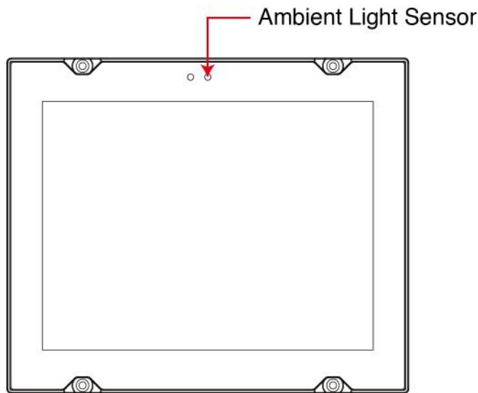
This sensor helps automatically adjust the brightness of the panel with the ambient light condition. The light sensor index is divided into 8 levels from L1 to L8; the lower the sensor index, the darker the panel. The panel brightness index is divided into 10 levels from 1 to 10, the lower the number, the darker the panel.
