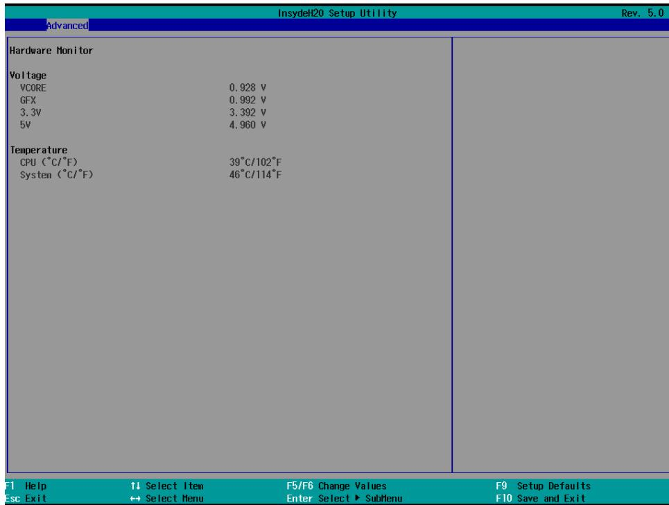
Note that the voltage values vary depending on the model. The temperature readings shown on the screen are within ±5% of the actual readings. However, the temperature readings are only valid when the ambient temperature is above 0°C.
