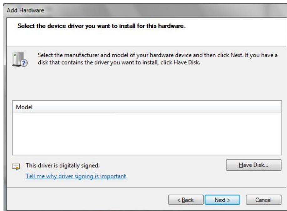
6. Point to the path **Driver\MPG-2101-W7E\_V1.0\_Driver\_Peripheral\4.MxGeneralIO\x64** and select **MxGeneralIo.inf**.
