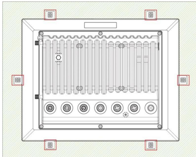
2. Use a torque of 4Kgf-cm to fasten the mounting screws and secure the panel-mounting kit onto the wall.
