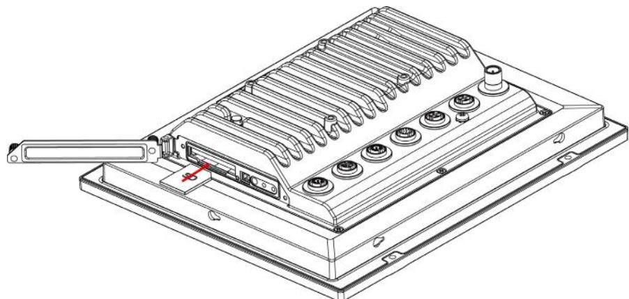
4. Reattach the cover and secure it with screws.
