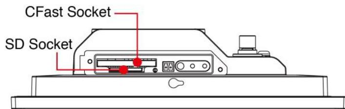
3. Insert the CFast or SD card into the slot using the push-push mechanism.
