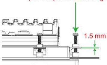
Ensure that there is adequate space behind the panel for ventilation, and that the panel material and thickness can support the weight of the device.
