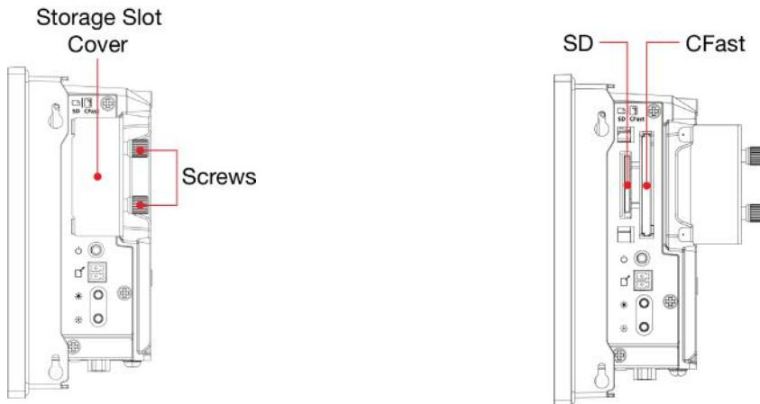
3. Reattach the cover and secure it with screws.
