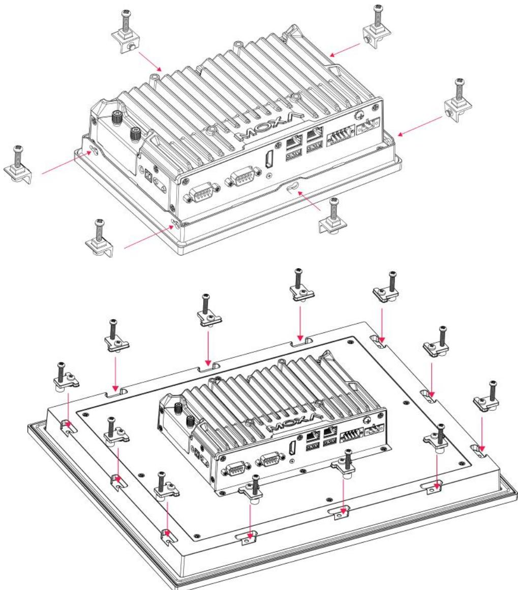
Use a torque of 5 kgf-cm to secure the mounting screws to fasten the panel-mounting kit onto the wall.
