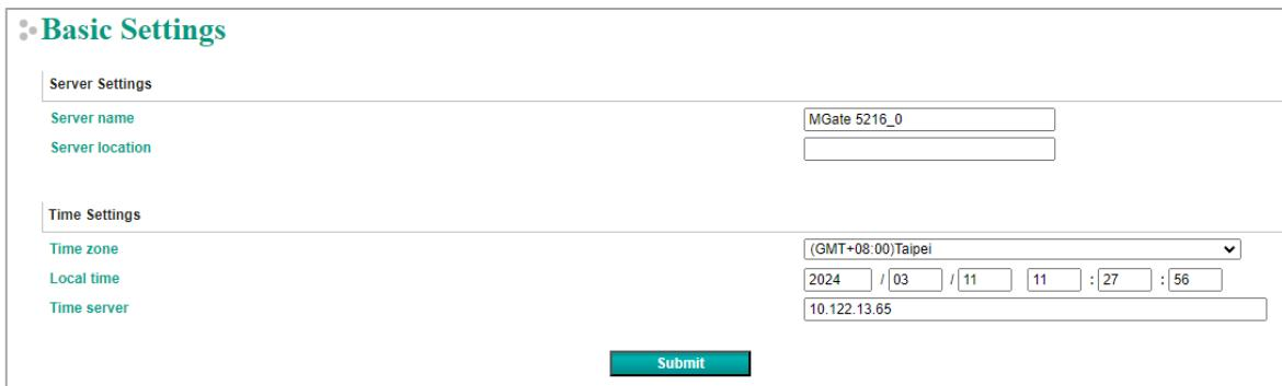
The screenshot shows the 'Basic Settings' page with two main sections: 'Server Settings' and 'Time Settings'. In the 'Server Settings' section, there are fields for 'Server name' (MGate 5216\_0) and 'Server location'. In the 'Time Settings' section, there is a dropdown for 'Time zone' (GMT+08:00) and a date/time input field (2024/03/11 11:27:56) with a 'Time server' IP address (10.122.13.65). A 'Submit' button is at the bottom.
