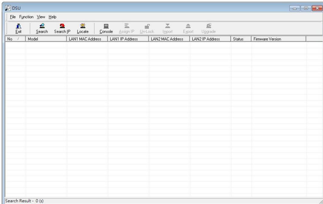
The DSU needs to connect to the unit before the unit can be configured. There are two methods to connect to the unit. **Broadcast Search** is used to find all MGATE 5111 units on the LAN. **Search IP** attempts to connect to a specific unit by IP address, which is useful if the unit is located outside the LAN or can only be accessed by going through a router.
