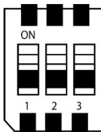
On the MGATE 5111's left side panel, you will find DIP switches to adjust each serial port's pull-up resistor, pull-down resistor, and terminator.
