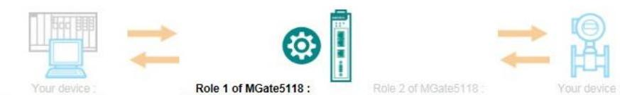
Role 1 of MGATE5118 : Modbus RTU/ASCII Master
