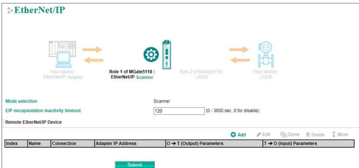
In **Scanner mode**, all EtherNet/IP connections will be shown in a table. For the initial setup, click **Add** to create a new connection.
