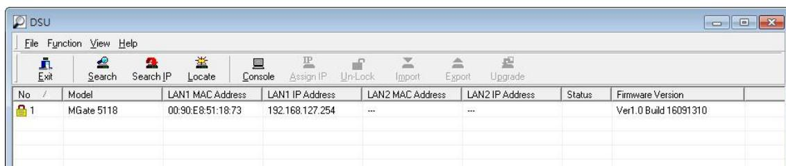
When the search is complete, every MGate 5118 found on the LAN will appear in the DSU window. The MAC address, IP address, and firmware version of each unit will be shown. Select the one you would like to configure.
