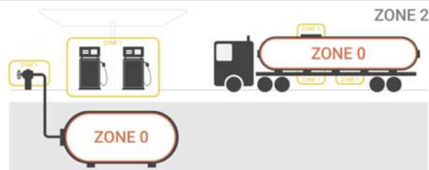
Figure 1: Zone Classification for Gas/Vapor/Mist
